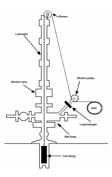
FIGURE 1 Schematic diagram of the arrangement during wireline operations.
