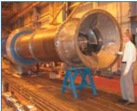
Figure 1. Zeron 100 seawater pump supplied to BOC to handle seawater with a high solids burden (up to 50,000mg/l)
