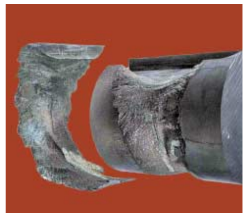
Fig. 5: Corroded and fatigued alloy K-500 shaft
