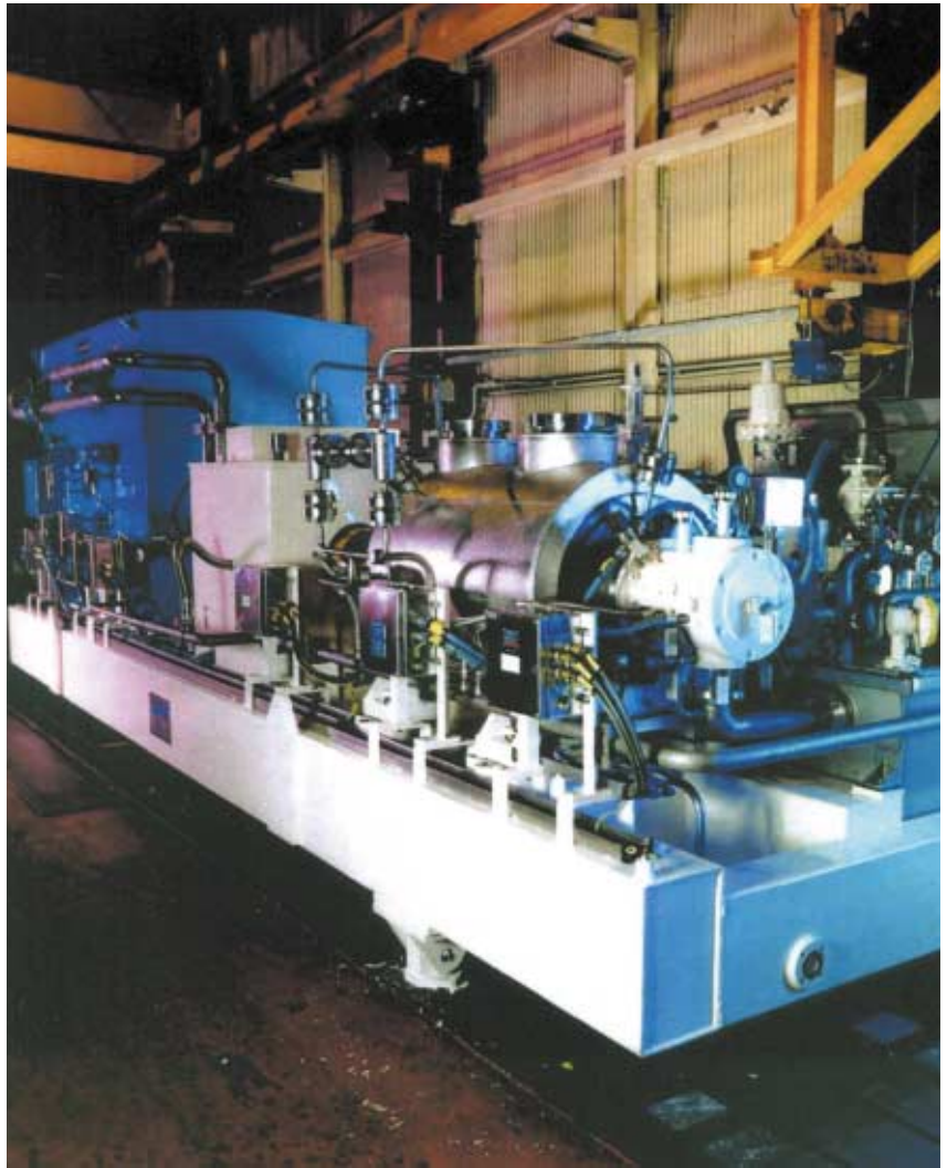
Fig. 3: Injection pump in Zeron 100 for the North Sea
