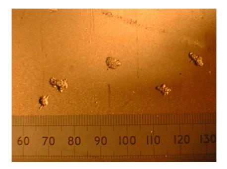
FIGURE 5 Appearance of pits on super duplex stainless steel from a HPAL heater
