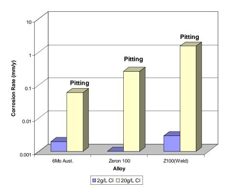
FIGURE 4 Corrosion rate in a simulated flash tank slurry at 100°C
