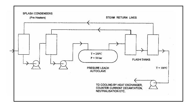
FIGURE 1 Schematic diagram of a HPAL circuit
