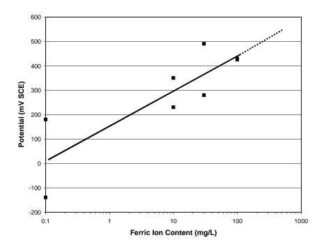
FIGURE 7 Potential of Zeron 100 versus ferric ion content in 10g/L chloride solution at pH2 and 90°C
