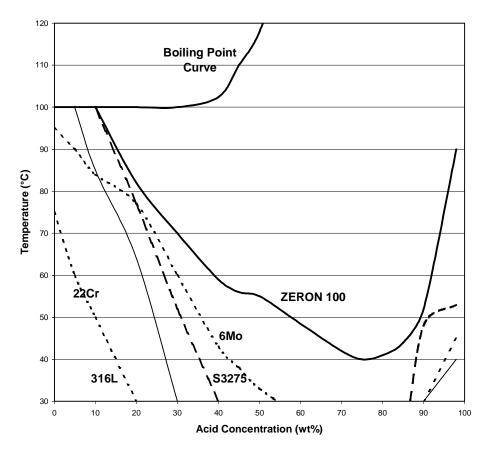
FIGURE 2 Iso-corrosion curves (0.1mm/y) for some stainless steels in sulphuric acid
