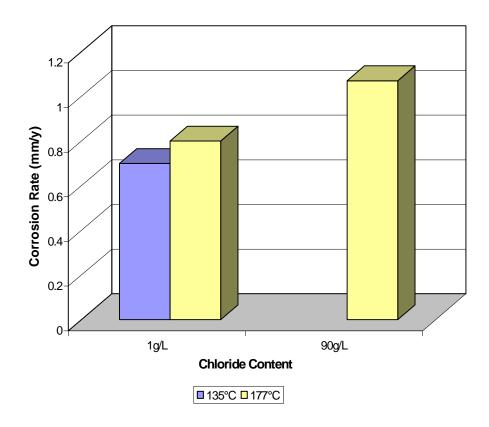
FIGURE 3 Corrosion rate of Zeron 100 in a simulated flash tank slurry
