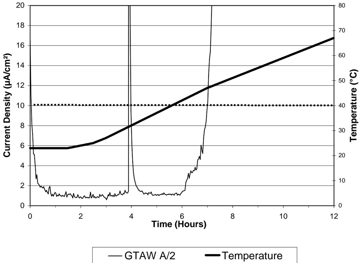
**FIGURE 2 Current versus time curve for welded super duplex stainless steel in sea water at +600mV SCE**
