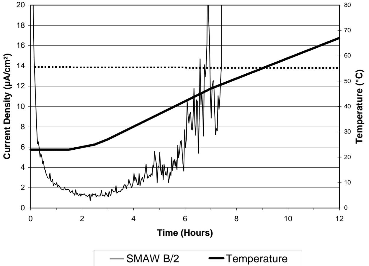
**FIGURE 3 Current density versus time during exposure at 600mV SCE in sea water at room temperature**
