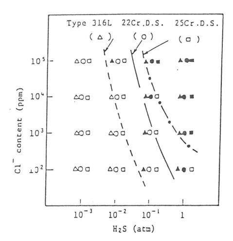
SCC susceptibility of 22Cr duplex stainless steel in Cl -H<sub>2</sub>S environtemt. O: No SCC, •: SCC (SSRT method: 80°C, strain rate 4.2 x 10<sup>-5</sup>/S)
