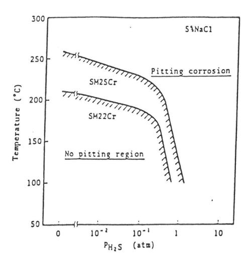
FIGURE 1: PITTING OF 22 Cr AND 25 Cr DUPLEX STAINLESS STEEL AS A FUNCTION OF  $\rm H_2S$  PRESSURE AND TEMPERATURE
