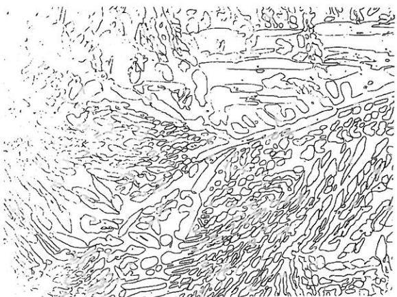
FIG. 1 - Microstructure of Cast and Heat Treated Zeron 25. Magnification X80
